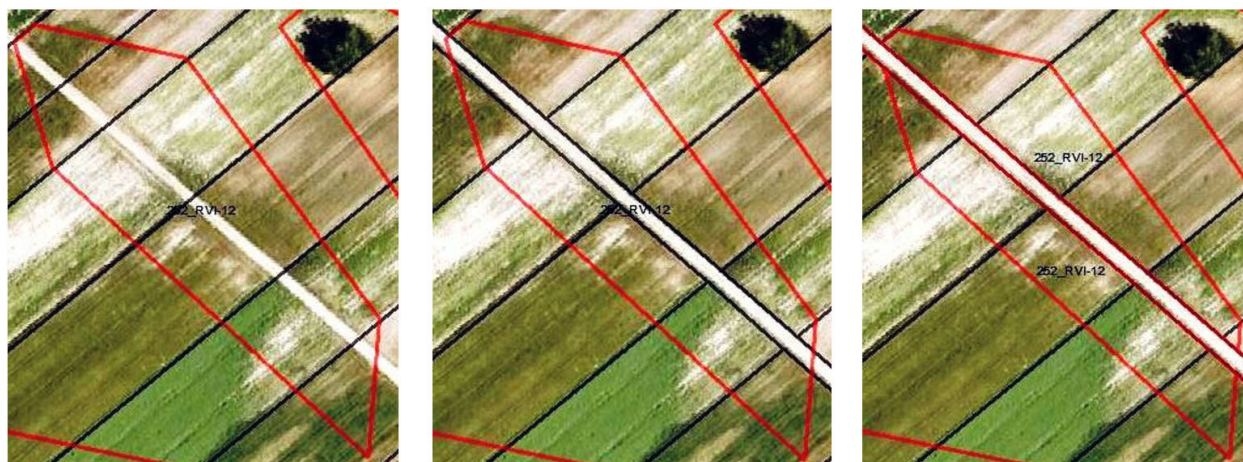
Fig. 4. Error correction in the land-use layer. Improvement of the land-use layer (red colour) to the parcel layer (black colour) Source: own elaboration.
