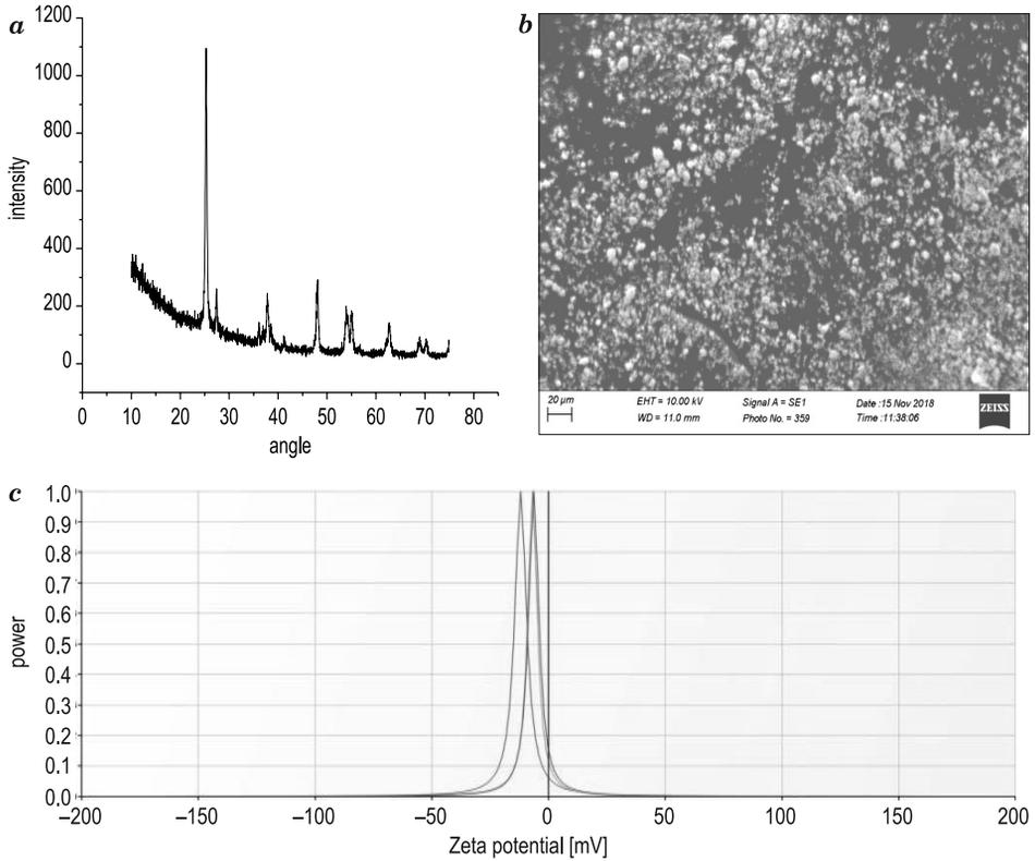
Fig. 1. Characterization of titanium dioxide nanoparticles (TiO<sub>2</sub> NPs): a – X-ray diffraction pattern; b – Scanning electron micrograph; c – Zetapotential of 1 mg L<sup>-1</sup> TiO<sub>2</sub> NPs. Scale bar represents 30 μm. Images at a magnification of 2000× in culture medium. Scale bar 10 μm. Images at a magnification of 2000×
