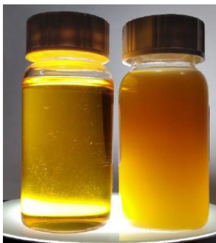
Fig. 1. TN-669 oil without water molecules (left) and containing water molecules (right) Source: based on NIDZGORSKA et al. (2023).
