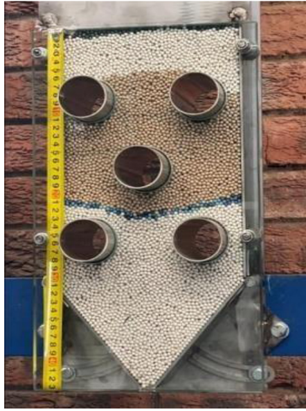
Fig. 6. The heat exchanger filled with particles Source: Drytech International (Pty) Ltd
