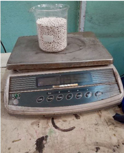
Fig. 3. Weighing the silicon particles Source: Drytech International (Pty) Ltd
