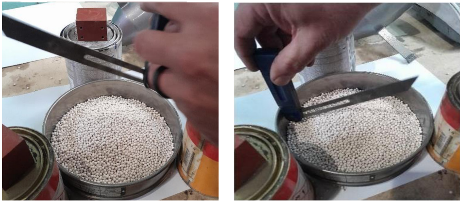
Fig. 4. Measuring the angle of repose Source: Drytech International (Pty) Ltd
