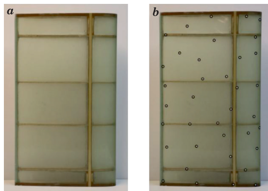
Fig. 7. Ready-to-test model: a – after removal from the mould and cutting off the excess material, b – after wrapping with paper reference points
