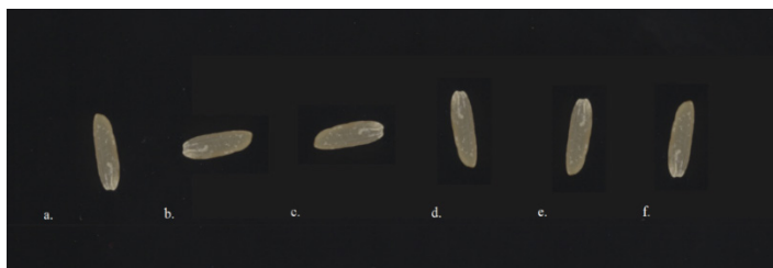
Fig. 5. Translation image of a natural rice grain with a variable angle of position: a – basic position, b – 90° rotation to the right, c – 90° rotation to the left, d – 180° rotation, e – vertical rotation with respect to the axis of symmetry, f – horizontal rotation with respect to the axis of symmetry
