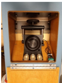
Fig. 6. Test stand for pycnometric volume measurement
