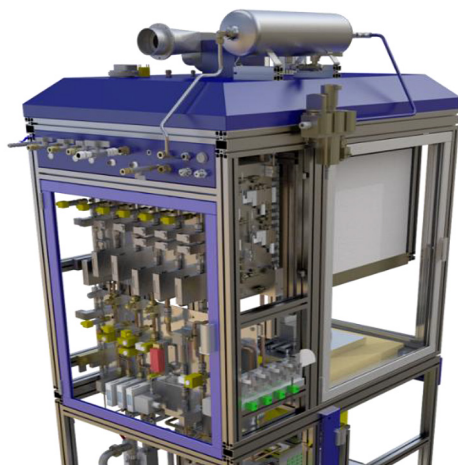
Fig. 5. Example of a Modular Measurement System for Individual Cells by EBZ GmbH Source: based on EBZ GmbH ( Test Rigs 2025).
