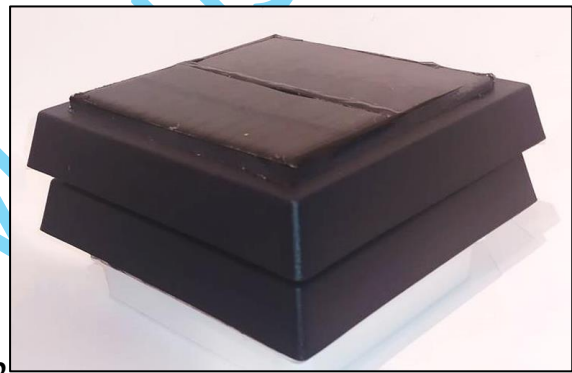
Fig. 5. 3D model of the mobile air quality monitoring station housing (a) and a photo of the assembled device (b) - a photovoltaic panel is visible on the top of the enclosure.
