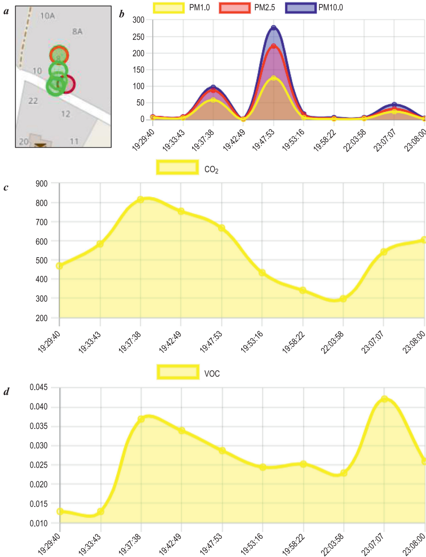
Fig. 10. The map showing the measurement points (a), and measurements of PM1.0/PM2.5/PM10 (b), CO 2 (c), and VOC (d) levels in a proximity of a lit charcoal grill
