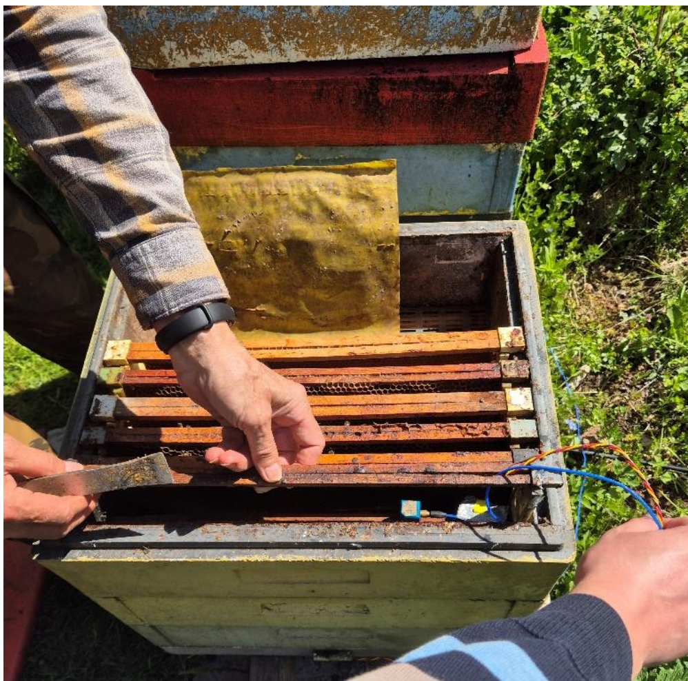
Figure 2: Apipol hive - placement of sensors
