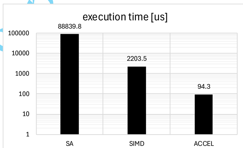
Fig. 5. Comparison of execution times for individual implementations (SA – Simple Algorithm, SIMD – Implementation using SIMD, ACCEL – Implementation using peripheral accelerator).
