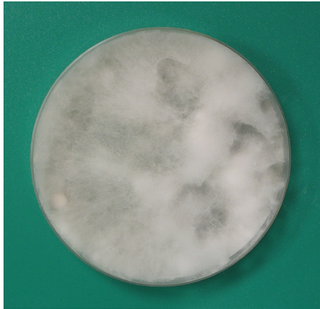
Fig. 3. Growth of fungi in composite after four months of storage in natural conditions
