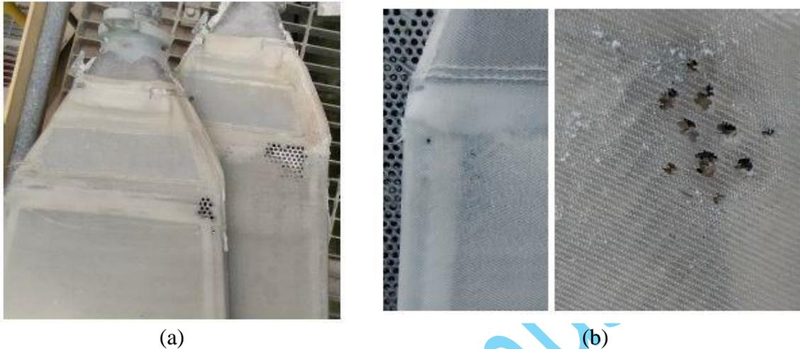
Figure 3: (a) Backing plates sector covered with a filtration membrane. (b) Failure condition of fabric, (Drytech Int.)
