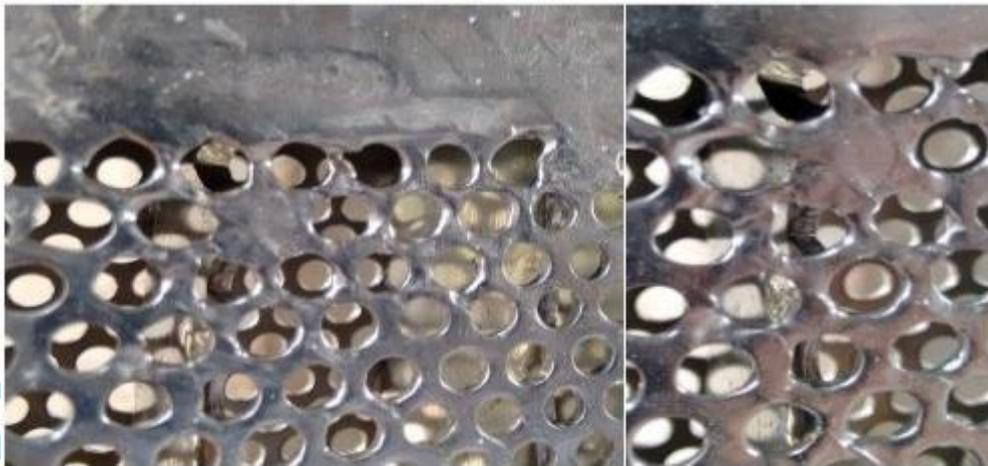
Figure 4: Damage to the sector backing plate, (Drytech Int.)
