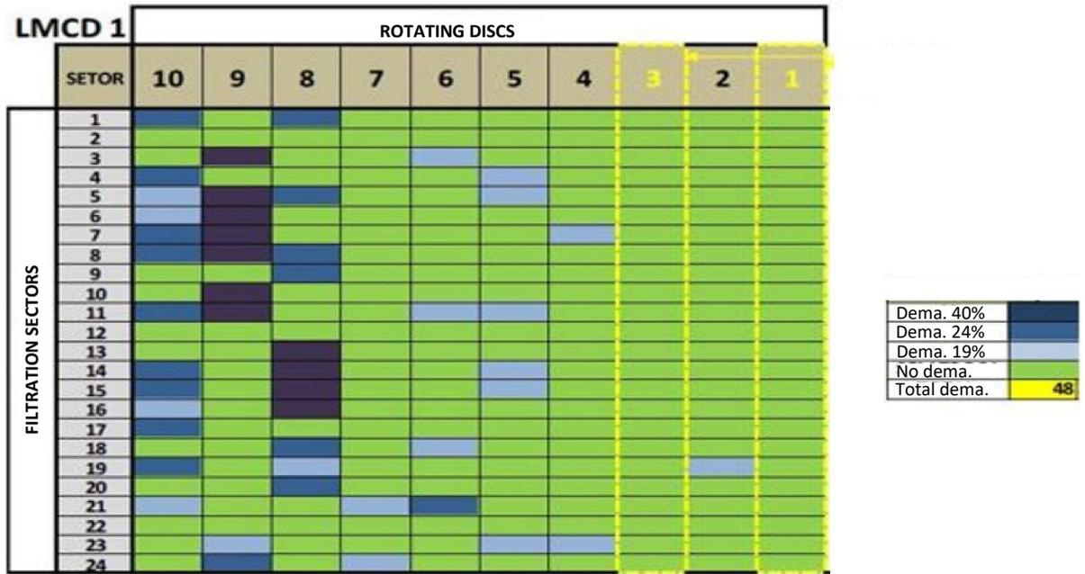
Figure 5: Location of material destruction in different disc's sectors, (Drytech Int.)
